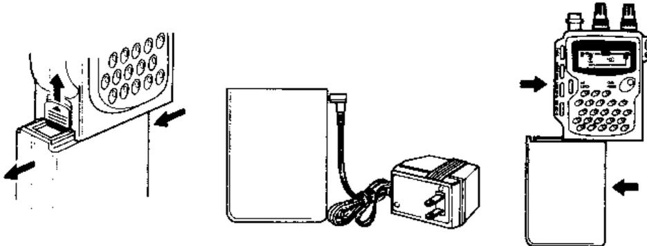
To charge the "AA" Ni-Cad batteries using the plug in Wall Charger:
