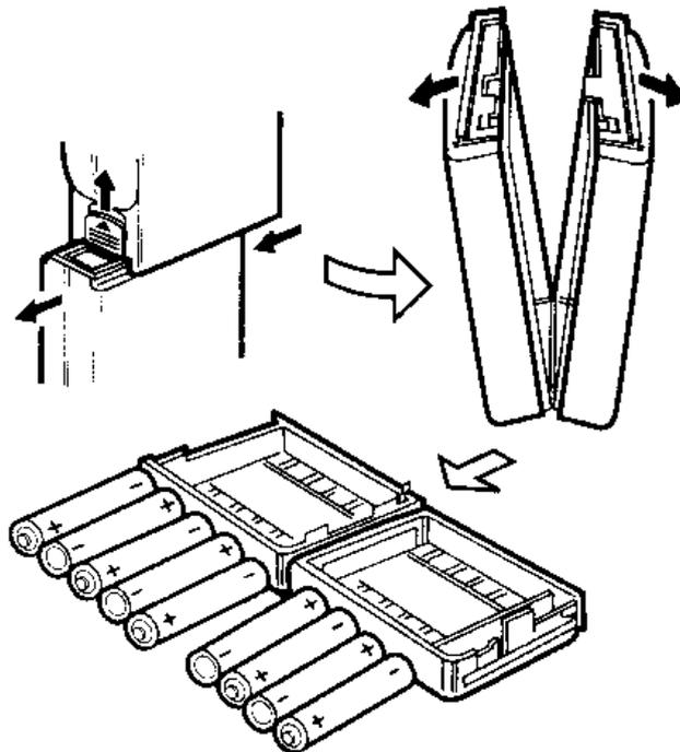
**IMPORTANT** When the batteries voltage become low, in addition to the "Battery Low" indicator coming on the display, you will experience a BLANK DISPLAY when you press the PTT button. This is due to the needed voltage being greater than the power you have left in the battery pack. This "Blank Display" situation is a normal reaction to the batteries becoming low. Please replace or re-charge to batteries immediately when this situation occur.
