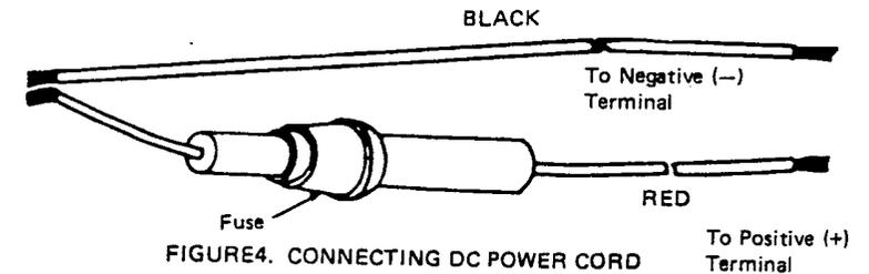
FIGURE 4. CONNECTING DC POWER CORD
